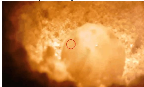
Fig. 2 Carbothermal reduction using concentrated optical energy
